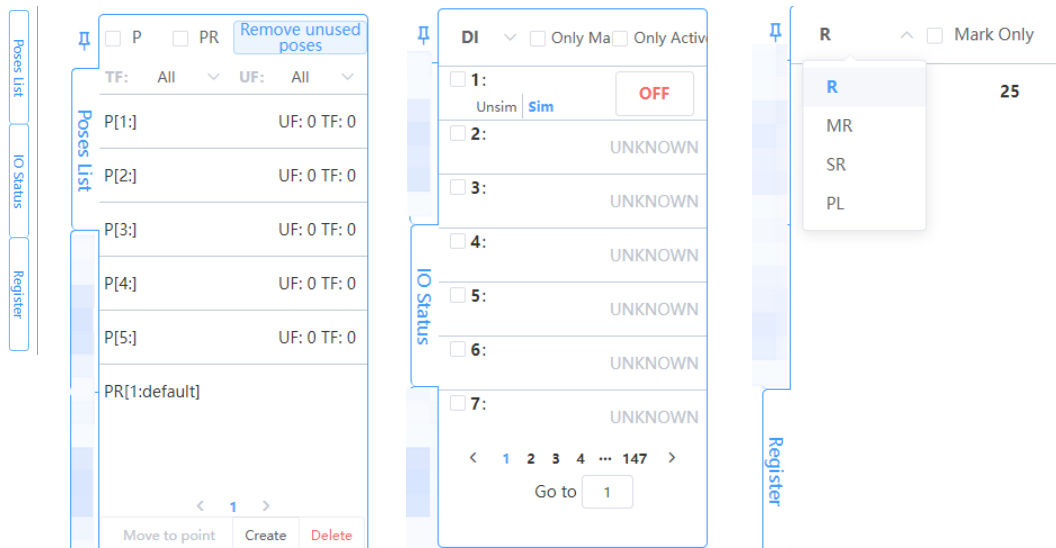
Fig. 4.5 shows the pose list, I/O status list and register list from left to right.
